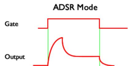
Gated Looping will trigger the ATTACK stage when the GATE goes high, then continue looping whilst the GATE remains high, and will RELEASE to zero when the GATE goes low.
